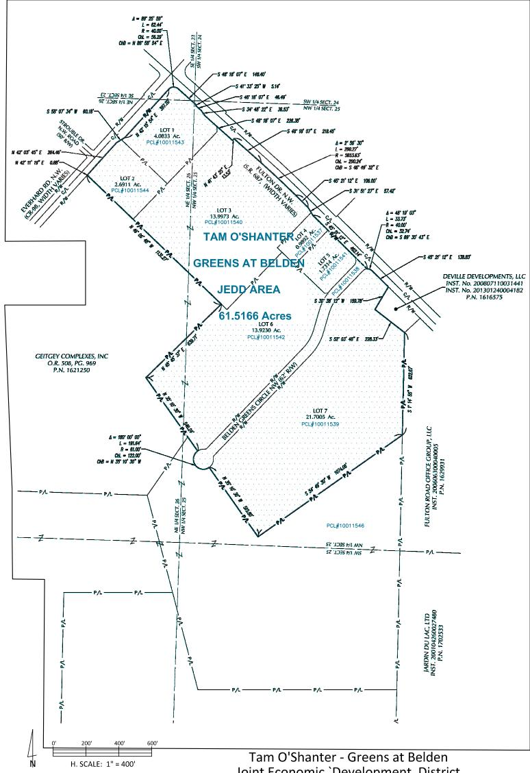
Basis of Bearing: Grid North of the Ohio State Plane Coordinate System, North Zone, NAD83(2011)
